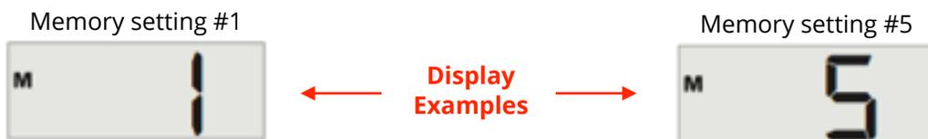
**Step 4:** Press the Menu button ( ● ) to store the value. The display will confirm by flashing 3 times.
